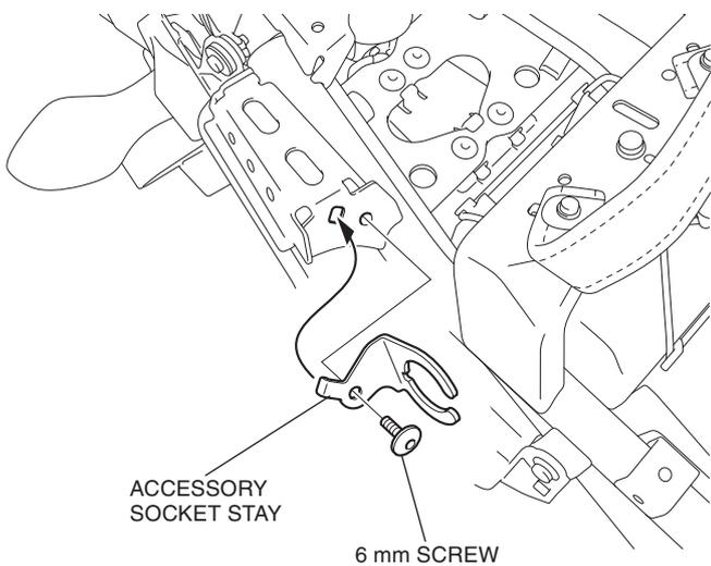
9. Install the accessory socket to the accessory socket stay as shown.
