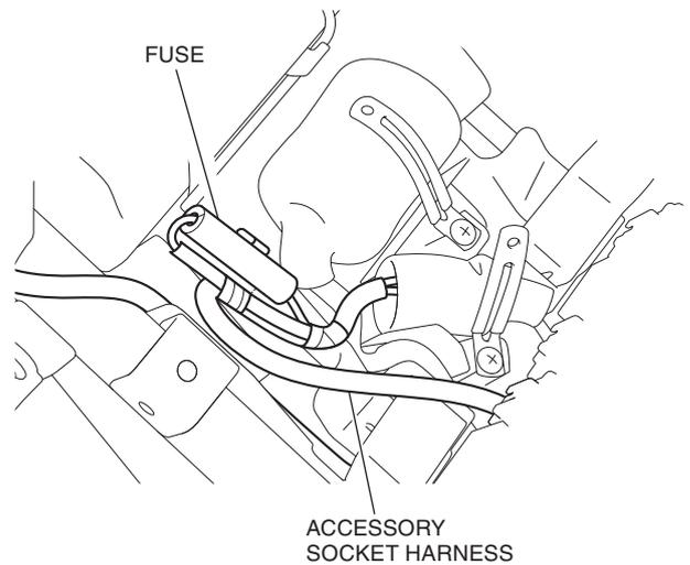
15. Secure the accessory socket harness with the wire ties as shown.
