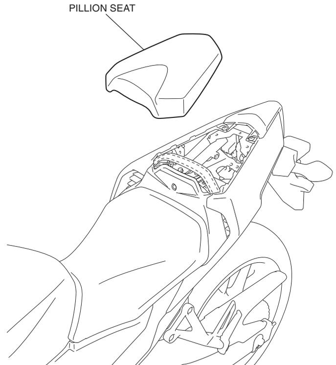
2. Remove the seat, and disconnect the negative (-) battery cable.
