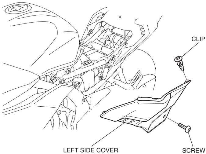
4. Remove the clips and screws as shown.
