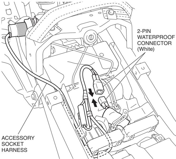
12. Secure the accessory socket harness with the wire tie as shown.
