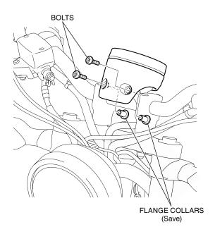
3. Refer to the Service Manual for the motorcycle, remove the headlight mounting bolts.
