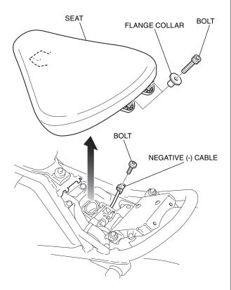
2. Refer to the Service Manual for the motorcycle, remove the bolts and collars as shown.
