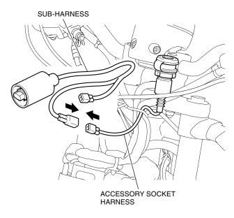
10. Remove the dummy connector as shown.
