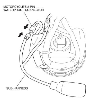
12. Secure the sub-harness with the wire tie as shown.
