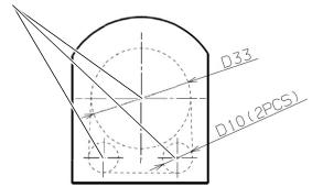
8. After drilling the holes, use a rotary tool and carbide burr to connect the circles by cutting along the dotted line, making a window.
