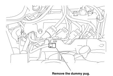
Install the accessory sub harness to the Red 4-pin connector and secure it to the clip/holder. Secure the sub-harness with the provided wire tie as shown.
