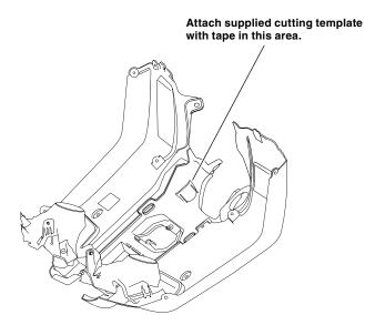
7. Drill the large hole with a 1-5/16 inch (33 mm) hole saw at the indicated mark.
