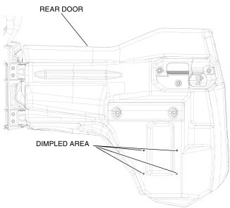
2. Install the drink holder with four trim clips through the holes drilled in Step 1 as shown.
