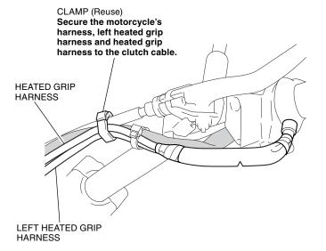
62. Secure the right heated grip harness with the wire ties as shown.
