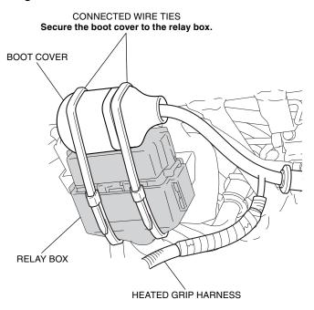
48. Secure the heated grip harness with the wire tie as shown.
