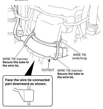
58. Secure the heated grip harness with the wire tie as shown.
