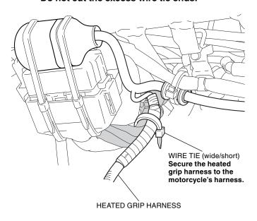
50. Pass the tube through the heated grip harness as shown.
