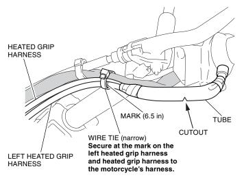
61. Secure the heated grip harness and left heated grip harness with the clamp as shown.
