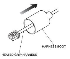
38. Connect the controller as shown.
