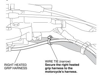
63. Secure the right heated grip harness with the wire tie as shown.
