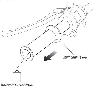
22. Using isopropyl alcohol, remove all traces of adhesive from the left handlebar.
