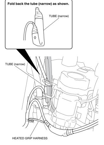
56. Secure the heated grip harness with the wire tie as shown.
