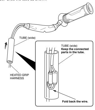
31. Secure the tube with electrical tape as shown.
