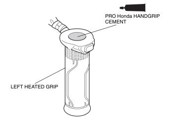
34. Apply Pro Honda Handgrip Cement to the left handlebar as shown.
