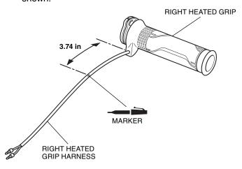
13. Install the clip band on the marked position as shown.
