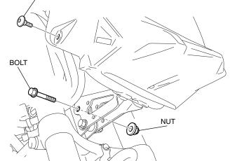
8. Loosen the nut and move the front upper cowl as shown
