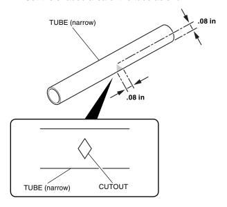
25. Pass the tube and cut tube over the heated grip harness as shown.
