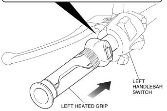
37. Pass the harness boot through the heated grip harness as shown.
