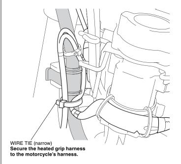
59. Secure the heated grip harness and left heated grip harness with the wire tie as shown.
