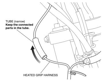
53. Secure the tube with electrical tape as shown.
