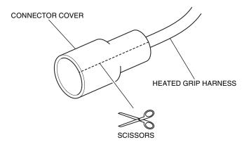
43. Remove the connector cover as shown.
