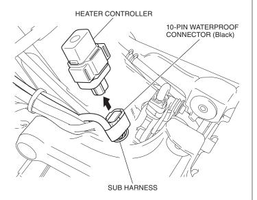
63. Install the heater controller as shown.
