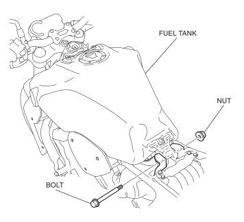
14. Remove the fuel tank as shown.
