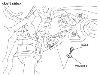
12. Remove the indicated parts by raising the front part of the fuel tank.
