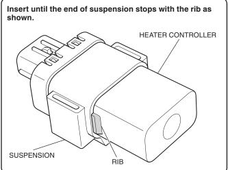
62. Connect the heater controller as shown.
