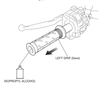
17. Using isopropyl alcohol, remove all traces of adhesive from the left handlebar.
