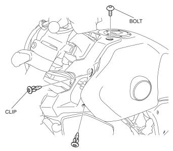
10. Remove the tank front cover as shown.
