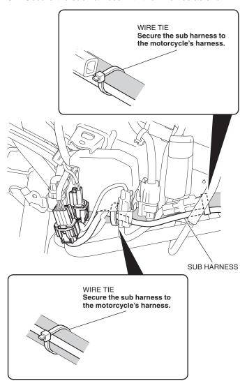
52. Secure the sub harness with the wire ties as shown.
