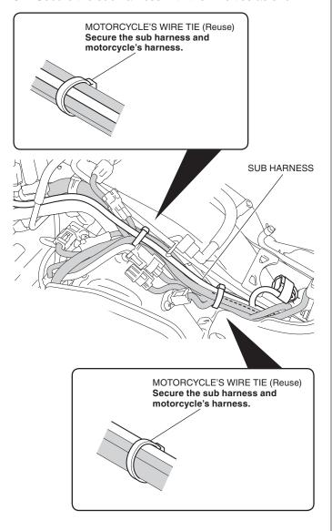
53. Secure the sub harness with the wire ties as shown.
