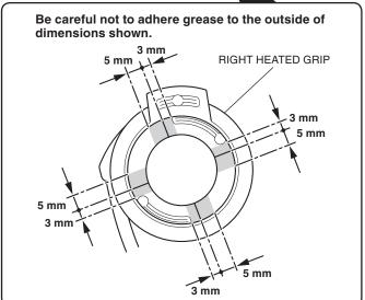
29. Apply grease to the hatched part as shown.
