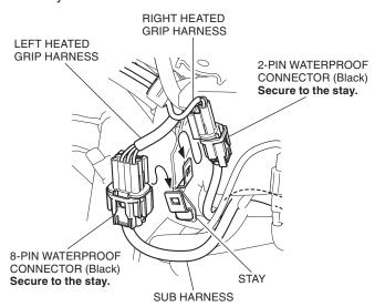
51. Secure the sub harness with the wire ties as shown.
