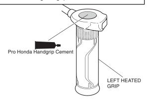
19. Apply Pro Honda Handgrip Cement to the left handlebar as shown.
