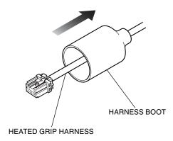
25. Connect the controller as shown.
