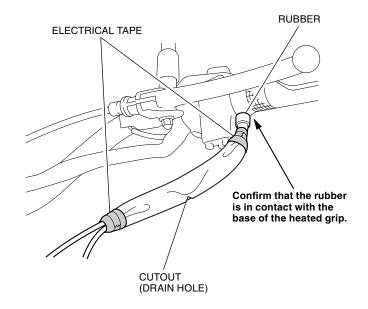
34. Secure the heated grip harness with the wire tie as shown.
