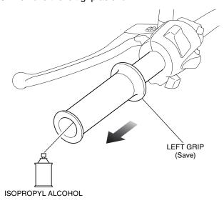
17. Using isopropyl alcohol, remove all traces of adhesive from the left handlebar.
