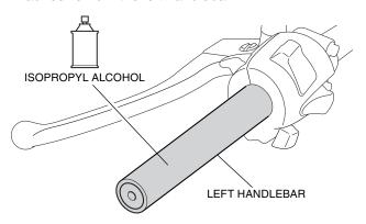
18. Liberally apply Pro Honda Handgrip Cement to the inside of the left heated grip as shown.
