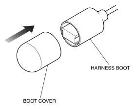
28. Secure the boot cover with electrical tape as shown.
