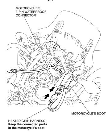
41. Secure the heated grip harness with the wire ties as shown.
