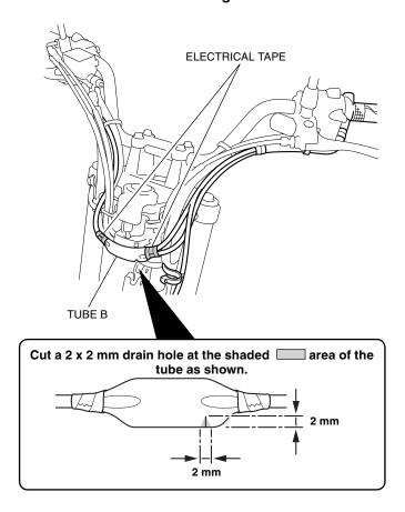
53. Secure the heated grip harness with the wire ties as shown.
