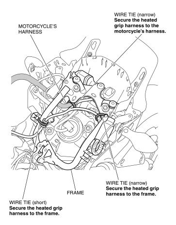
42. Pass the tube over each heated grip harness as shown.
