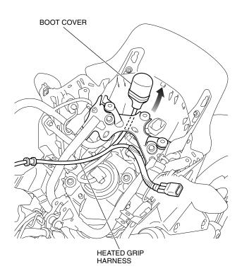
36. Secure the heated grip harness with wire tie as shown.
