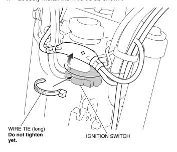
2. Secure each harness with the wire ties as shown.
