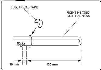
47. Pass the tube over the heated grip harness as shown.
