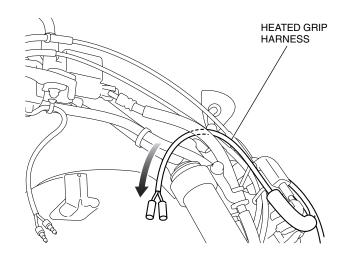
46. Bundle the right heated grip harness with electrical tape as shown.
