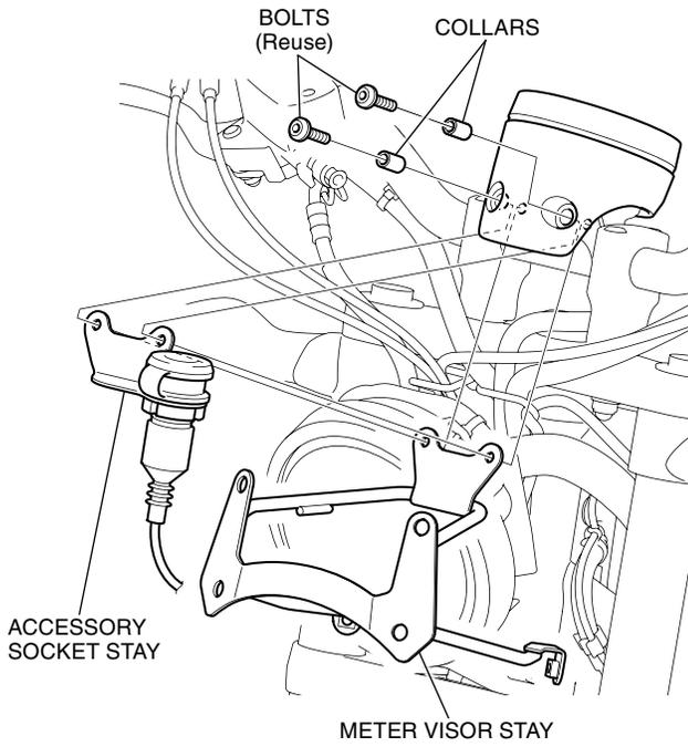
5. Tighten all loosely installed bolts to the value specified in the Torque Chart.
