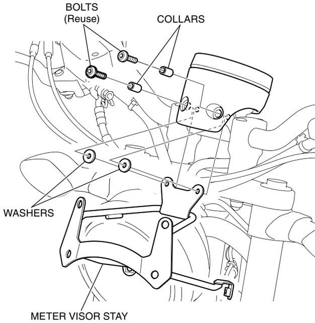
4. Loosely install the bolt as shown.
