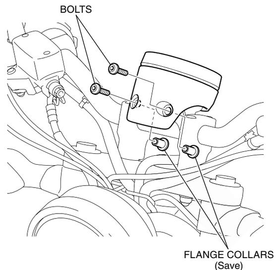
2. Refer to the Service Manual for the motorcycle, remove the bolt and nuts.
