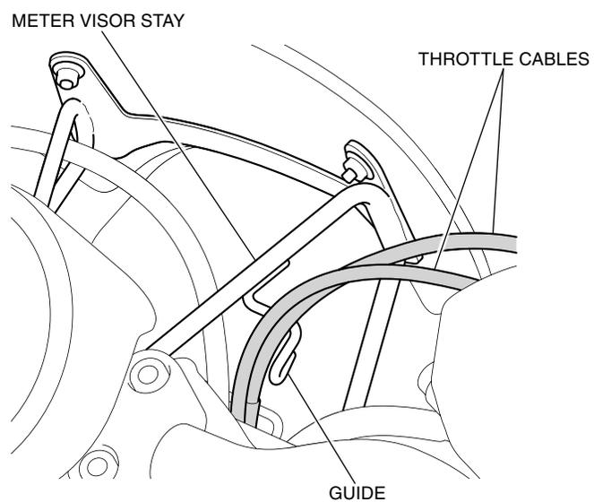
8. Move the handlebar right and left, and check that this accessory does not interfere with the motorcycle parts.
