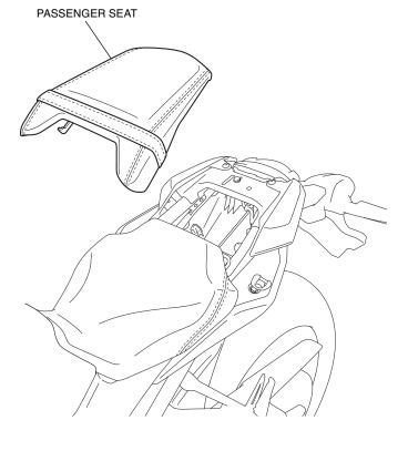
2. Remove the main seat and disconnect the negative (-) cable of the battery.
