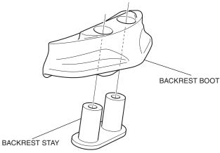
5. Install the assembled backrest as shown.
