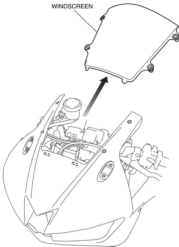
4. Remove the well nuts from the existing windscreen as shown.
