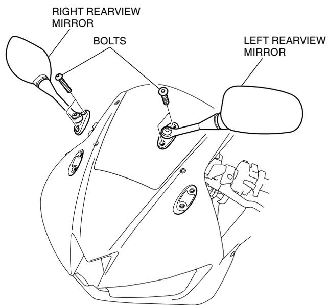
2. Remove the bolts and washers from the motorcycle as shown.
