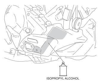
8. Peel off the adhesive backings on the right foot deflector as shown.
