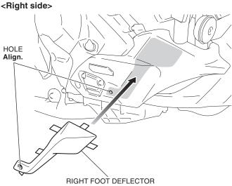
10. Remove the adhesive backings as shown.
