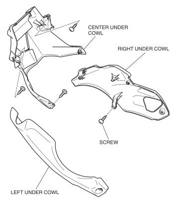
3. Cut and attach the templates to the under cowls and mark them using an awl as shown.
