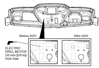
4. Install the horn switch into the hole in the instrument panel as shown.
