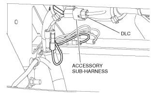
15. Secure the accessory sub-harness using one wire tie to the vehicle frame rail as shown.
