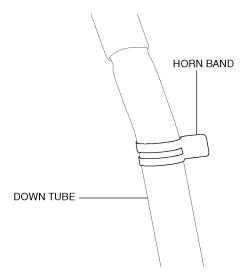
9. Install the horn at a 90 degree angle on the down tube. Connect the horn wire harness to the horn.
