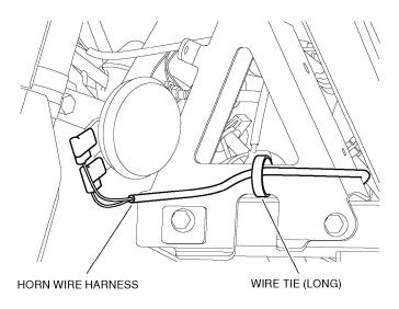
11. Remove the clip shown with care and avoiding wire damage.
