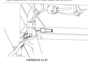
13. Connect the horn wire harness to the horn switch by matching the wire colors as shown.
