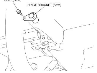
8. Loosely install the left hinge bracket as shown.
