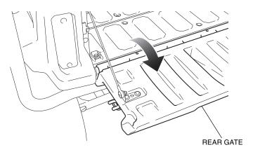
2. Remove the tie down hook as shown.
