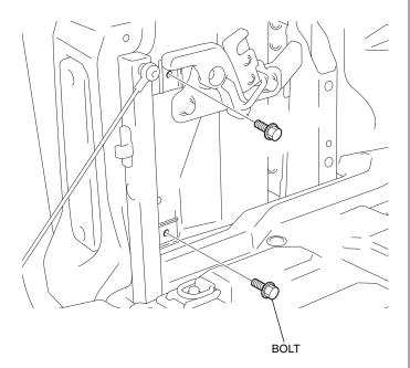
Remove the tie down hook as shown.
