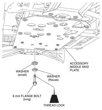
12. Tighten the loosely installed hardware to the values specified in the Torque Chart.
