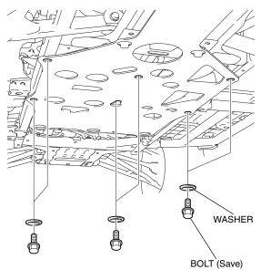
3. Remove the middle skid plate as shown.
