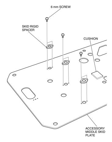
8. Install the skid rigid collar as shown.
