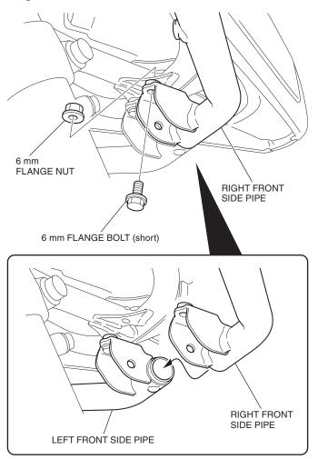
Install the 6 mm flange bolt (short) and 6 mm flange nut as shown.
