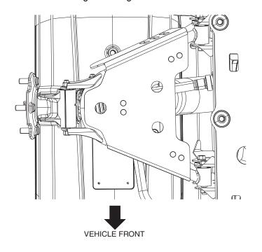
3. Insert two screws through the countersunk holes in the guard and assemble the bracket as shown.
