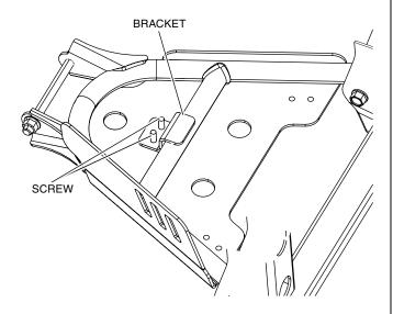
4. Thread a nut onto each screw and tighten until the bracket loosely contacts the guard.
