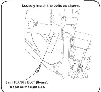
5. Loosely install the parts as shown.
