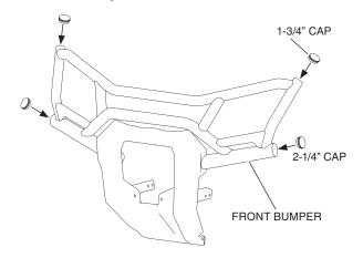
4. Loosely install the front bumper as shown.
