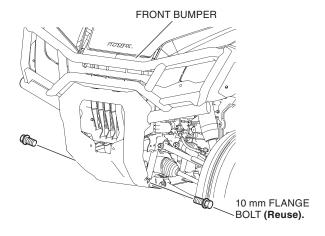
6. Tighten the loosely installed hardware to the values specified in the Torque Chart.
