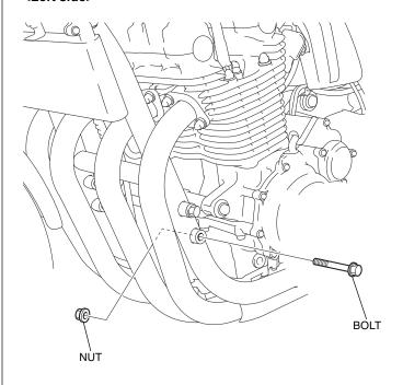
Loosely install the left engine guard as shown.
