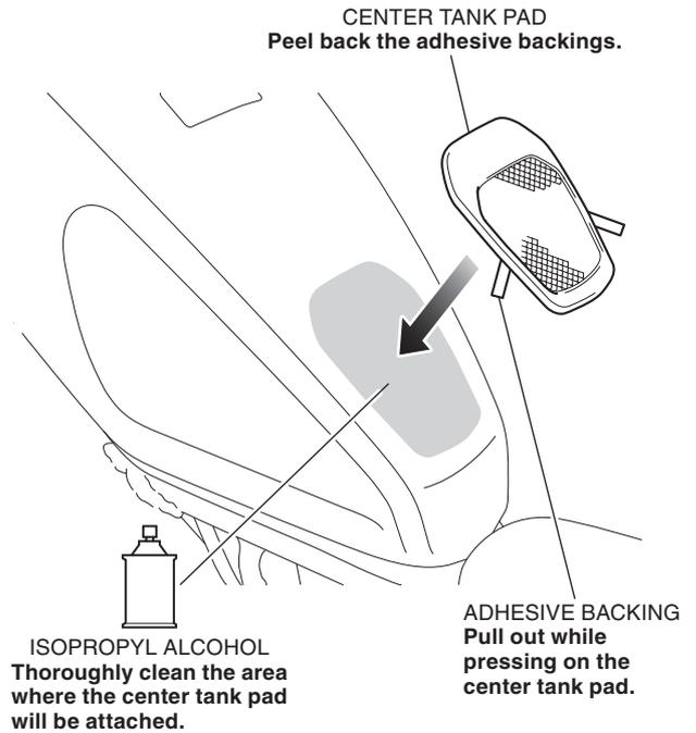
**Align the center of the fuel tank with the center of the center tank pad.**
