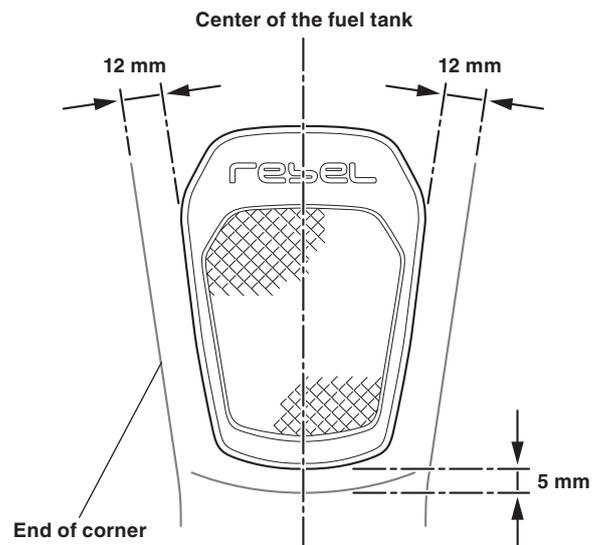
2. Apply adequate pressure to the attached center tank pad.
