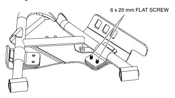
4. Thread a U-nut onto each screw and tighten until the bracket loosely contacts the guard.
