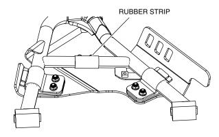
Assemble the bracket around the rubber strip as shown.
