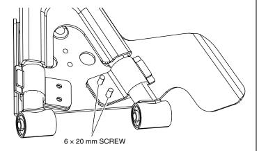
4. Thread a U-nut onto each screw and tighten until bracket loosely contacts the guard.
