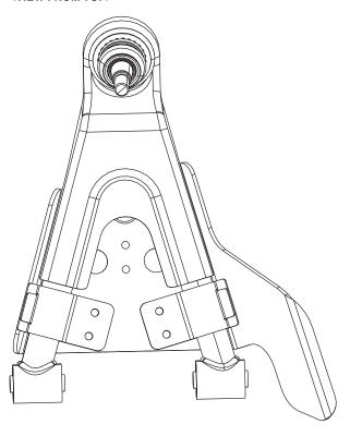
3. Pass two screws through the countersunk holes in the guard and assembled bracket as shown.
