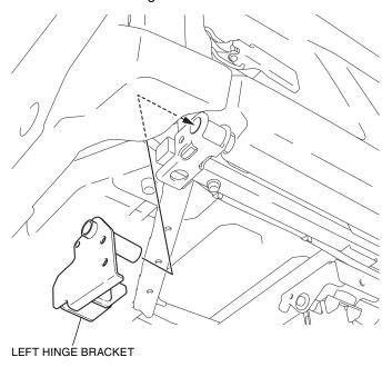
4. Loosely install the 6 mm flange bolt as shown.
