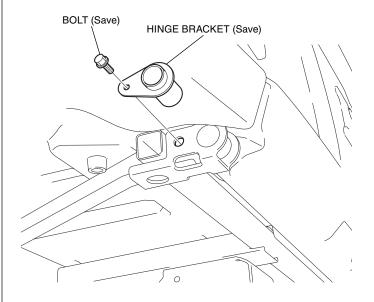
3. Install the left hinge bracket as shown.
