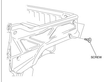
2. Remove the hinge bracket as shown.
