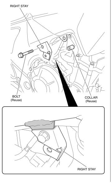
4. Remove the bolt and collar as shown.
