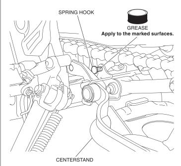
10. Install the spring plate as shown.
