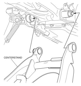
Install the circlip and washer as shown.
