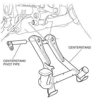
5. Install the 6 mm bolt and flange nut as shown.
