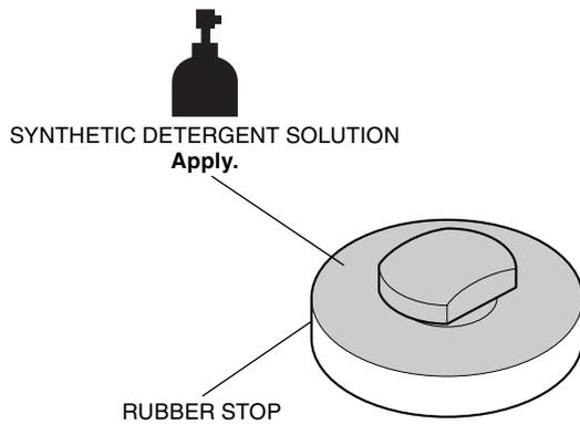
4. Install the rubber stop in the position shown.
