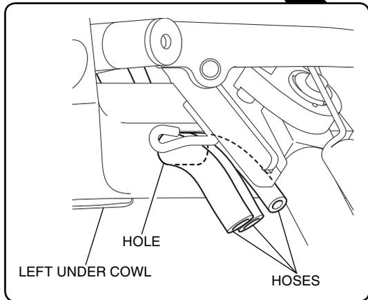
3. Apply synthetic detergent solution to the rubber stop in the area shown.
