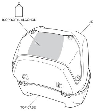
3. Peel off the adhesive backings on the rear of the top case lid panel as shown.
