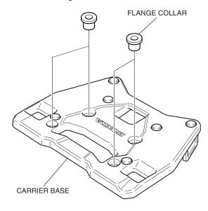
Install the carrier base as shown.
