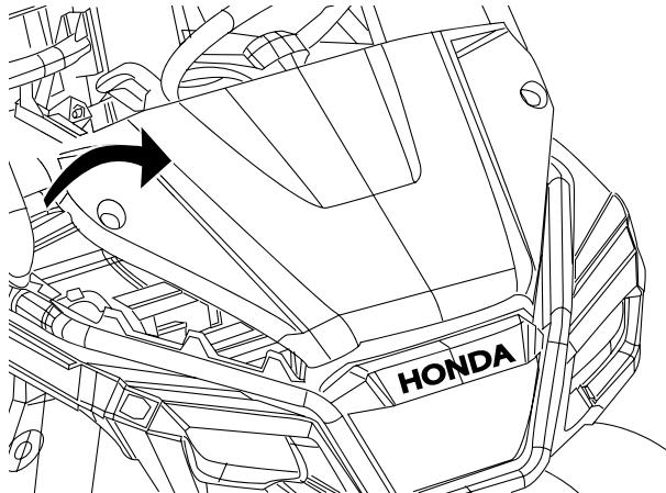
2. Place the underhood storage tray between the center of the frame tubes and mark the new fastener locations as shown.
