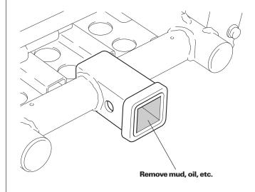
2. Install the receiver hitch cover plug as shown.
