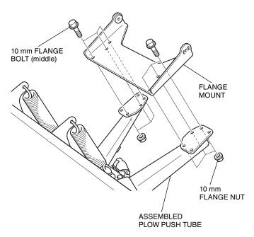
9. Install the assembled flange mount as shown.
