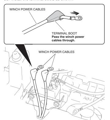
39. Install the winch power cables to the corresponding color terminal on the contactor as shown.
