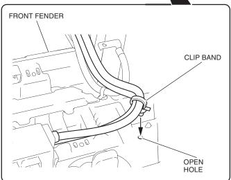
51. Secure the winch ground cable and sub harness with the wire tie as shown.
