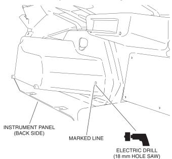
8. Position the remote control sub harness as shown and mark this position.
