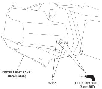
10. Open the glove box and pass the remote control sub harness through the hole in the instrument panel.
