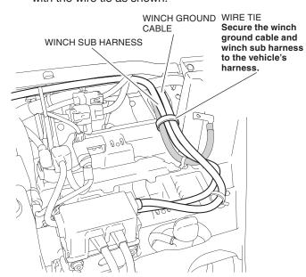
52. Secure the winch sub harness with the wire ties as shown.
