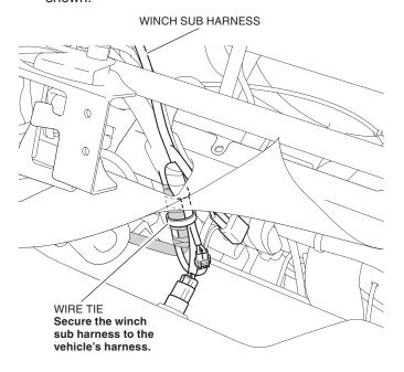
18. Connect the winch sub harness and remote control sub harness as shown.
