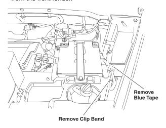
35. Route the winch power cables through the hole in the front fender as shown.
