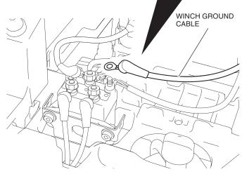
47. Install the winch ground cable as shown.
