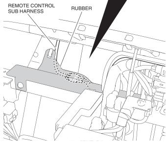
19. Secure the harnesses with the wire ties as shown.
