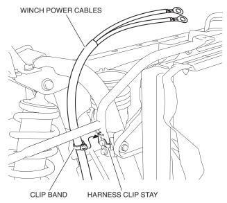
23. Secure the winch power cables with the wire tie as shown.
