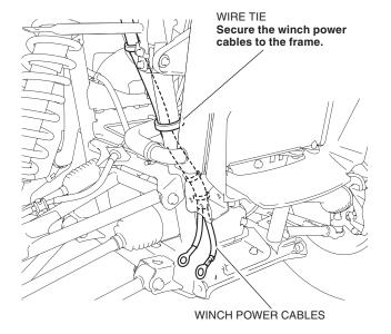
28. Install the winch power cables as shown.
