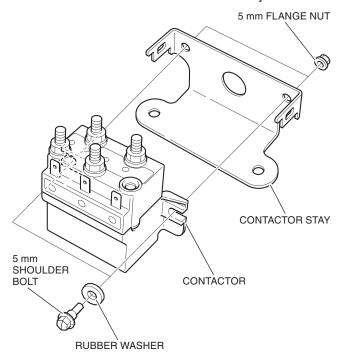
14. Install the assembled contactor to the front fender as shown.
