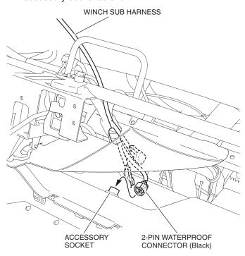
16. Connect the vehicle's harness to the winch sub harness as shown.
