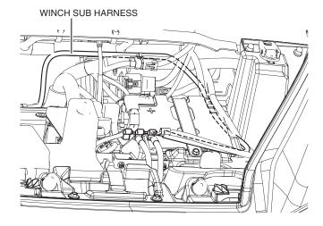
37. Connect the sub harness to the contactor as shown.
