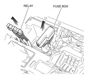
15. Remove the fuse holder and starter relay switch as shown.
