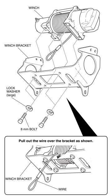
75. Loosely install the assembled winch as shown. **<Front side>**
