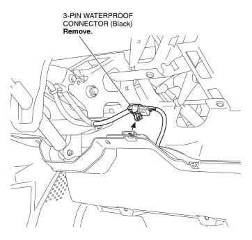
39. Remove the front floor cover as shown.
