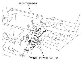
78. Route the sub harness and winch ground cable as shown.
