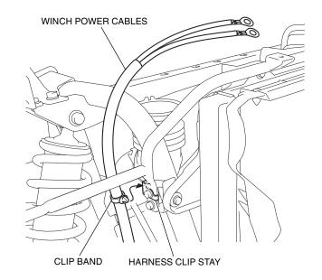
68. Secure the winch power cables with the wire tie as shown.
