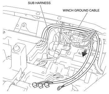
79. Connect the sub harness to the contactor as shown.
