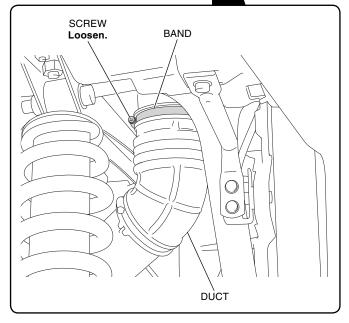
2. Remove the vehicle's parts as shown.
