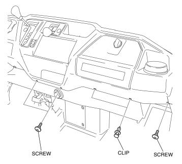
21. Remove the parts as shown.
