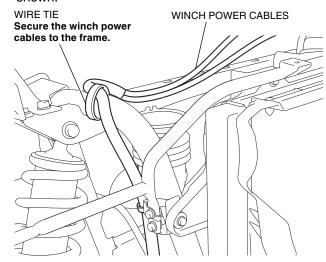
69. Secure the winch power cables with the wire tie as shown.
