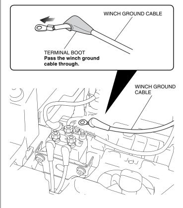
89. Install the winch ground cable as shown.
