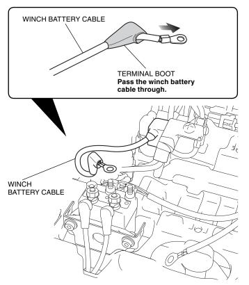
87. Install the winch battery cable as shown.
