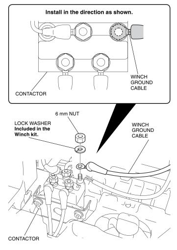
90. Cover each cable terminal with the terminal boot as shown.
