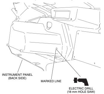
44. Position the remote control sub harness as shown and mark this position.
