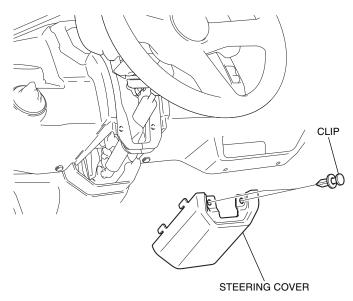
24. Remove the parts as shown.
