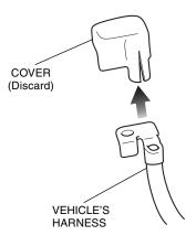
85. Connect the winch battery cable as shown.
