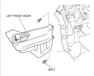
6. Remove the left front mud guard as shown.
