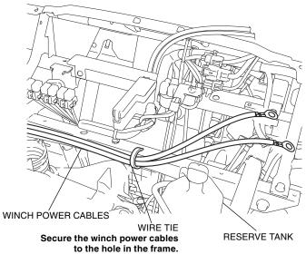
70. Route the winch power cables and secure it with the wire tie as shown.
