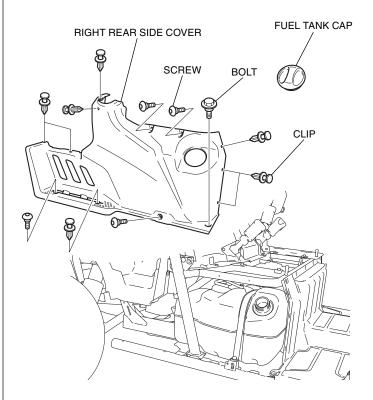
30. Install the fuel tank cap as shown.
