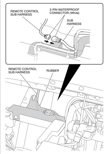
64. Secure the harnesses with the wire ties as shown.
