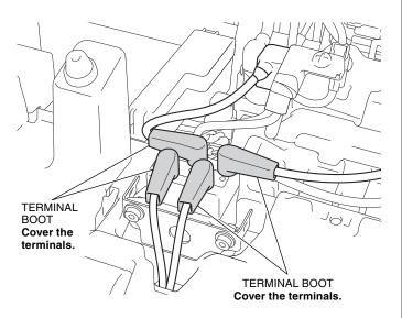
91. Install the contactor cover as shown.
