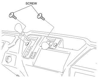
22. Remove the select lever knob and change lever knob as shown.
