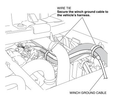
55. Route the winch ground cable and secure it with the wire ties as shown.
