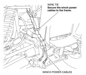
71. Install the winch power cables as shown.
