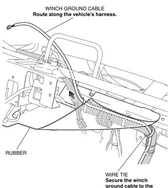
ground cable to the vehicle's harness.
