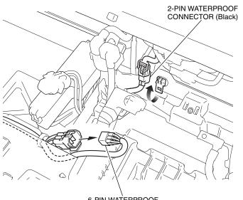
6-PIN WATERPROOF CONNECTOR (Black) 17. Remove the clips as shown.
