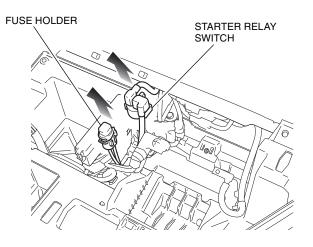
16. Remove the connectors as shown.
