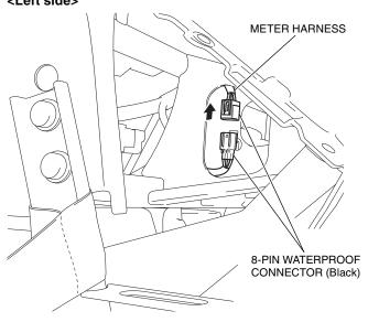
26. Remove the instrument panel as shown.
