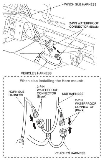
60. Connect the vehicle's harness to the winch sub harness as shown.
