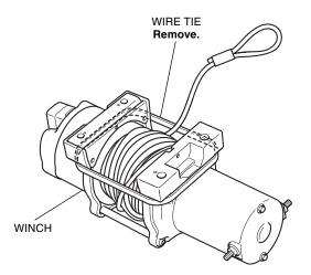
74. Install the winch to the winch bracket as shown.
