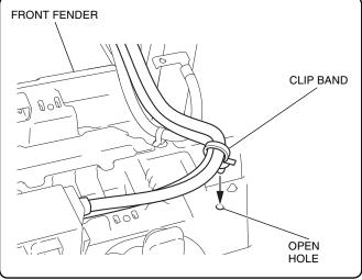
93. Secure the winch ground cable and sub harness with the wire tie as shown.
