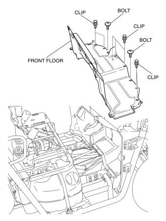
37. Remove the indicated parts as shown.
