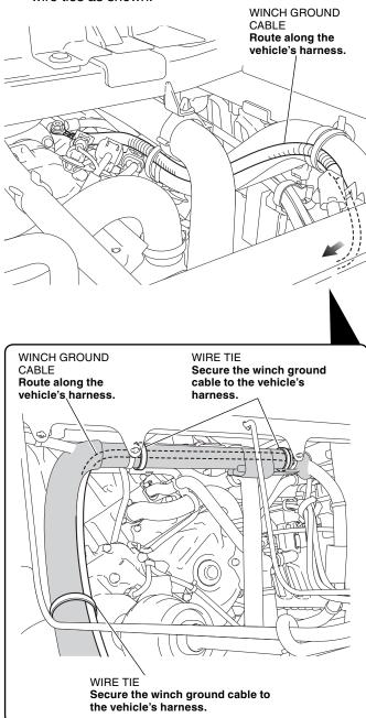
56. Route the winch ground cable and secure it with the wire ties as shown.
