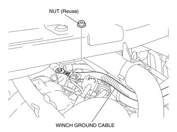
54. Secure the winch ground cable with the wire ties as shown.
