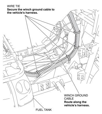
57. Route the winch ground cable and secure it with the wire tie as shown.
