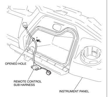
47. Install the remote control sub harness as shown.
