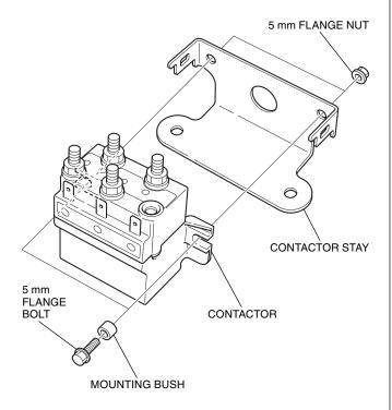
50. Install the assembled contactor to the front fender as shown.
