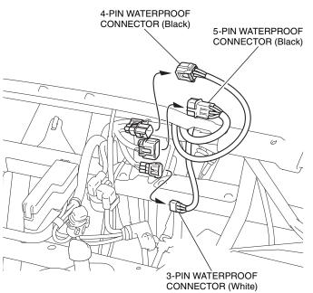
20. Remove the parts as shown.
