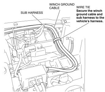
94. Secure the winch ground cable and sub harness with the wire ties as shown.
