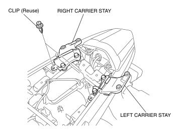
7. Install the rear carrier A as shown.
