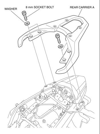
8. Securely tighten the bolts as shown.
