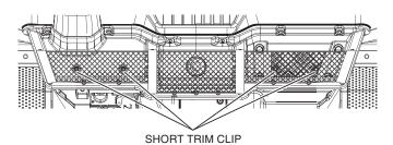
10. Install the passenger side storage net to the trim clips as shown.
