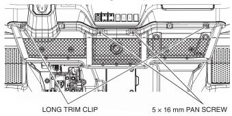
4. Apply upward pressure to hold storage unit assembly firmly against the floor cover panel. Use the holes shown as a template to mark the position of four holes to be drilled in the floor cover.
