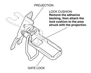
7. Install the left tail gate bracket and gate lock as shown.
