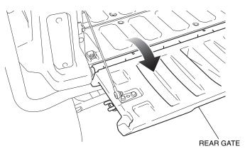
Remove the stopper wire as shown.
