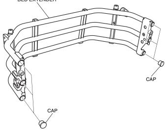
19. Install the bed extender on the left and right bed extender brackets as shown.
