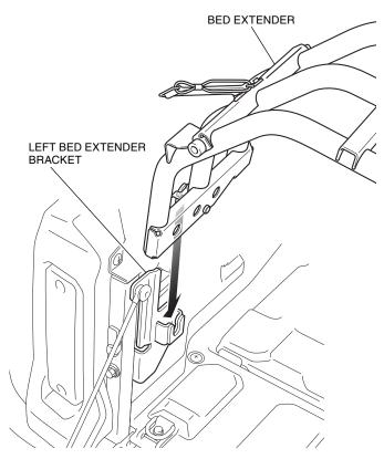
20. Bring the bed extender down and secure it with the band.
