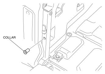
12. Loosely install the left bed extender bracket as shown.
