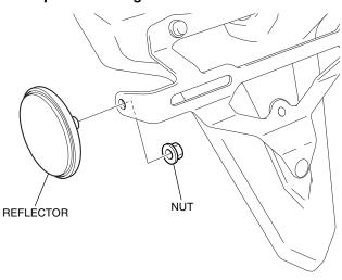
4. Install the reflector stay as shown.
