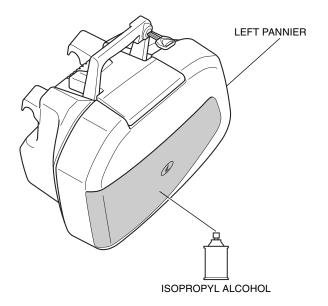
3. Peel off the adhesive backings on the left pannier cover as shown.
