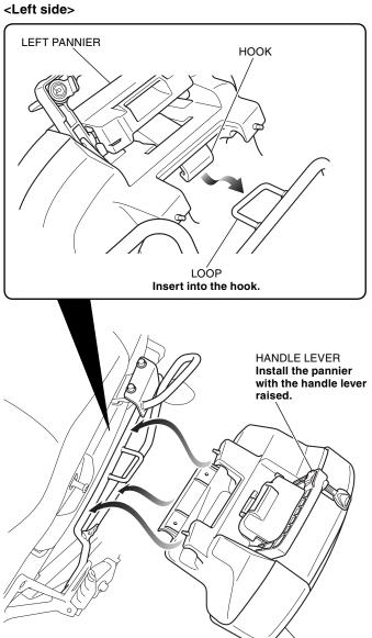
3. Lower the handle lever and lock the left pannier by turning the key counterclockwise as shown.
