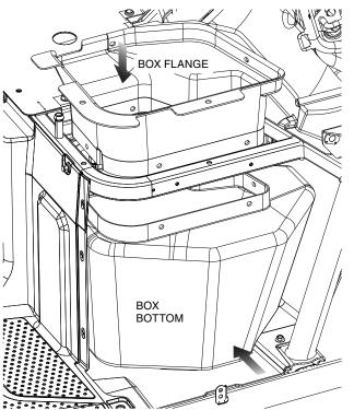
3. Align the holes between the box bottom and the box flange and connect them together with seven trim clips as shown.
