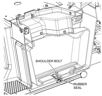
5. Referring to the Service Manual for the vehicle, re-install the seat and the left side cover using the original hardware set aside in Step 1.
