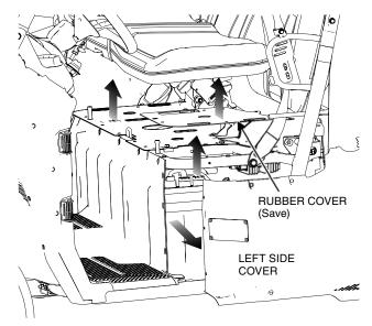
2. Slide the box bottom in from the side opening and insert the box flange through the opening under the seat.
