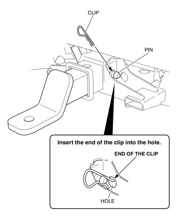
4. Install the trailer hitch ball as shown.
