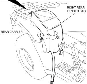
3. Raise the right rear fender bag as shown and remove the adhesive backing from the hook and loop tape as shown.
