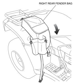
5. Route the belt as shown to secure the right rear fender bag.
