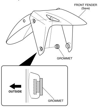
3. Install the accessory front fender in the reverse order of removal.
