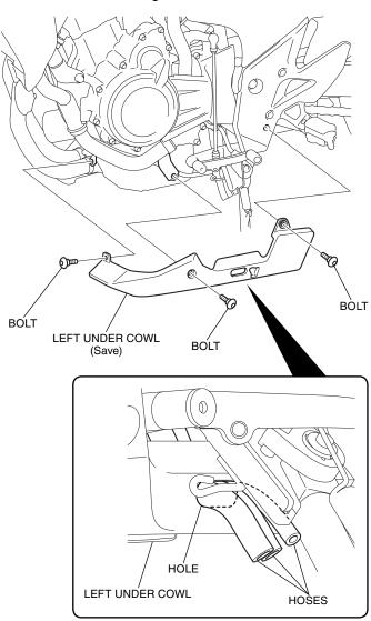
2. Install the accessory left under cowl in the reverse order of removal.
