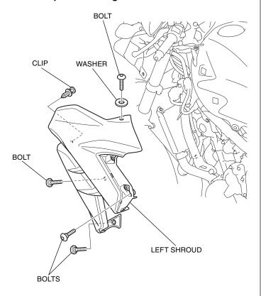
5. Refer to the Service Manual for the motorcycle, remove the left and right inner cowls.
