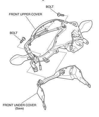
9. Exchange the front under cover for the accessory part as shown.
