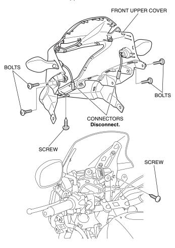
8. Remove the existing front under cover as shown.
