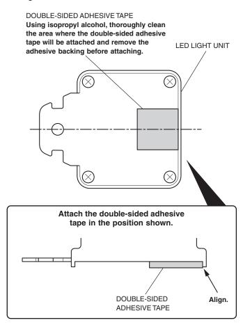
15. Install the lower spoiler stay and LED light unit as shown.
