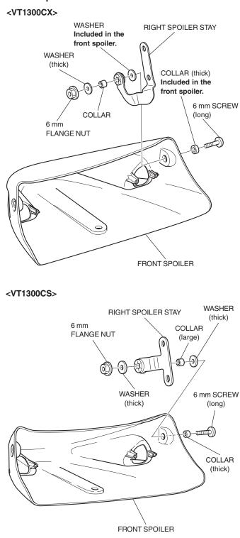
Install the LED light to the front spoiler as shown. Repeat on the other side.
