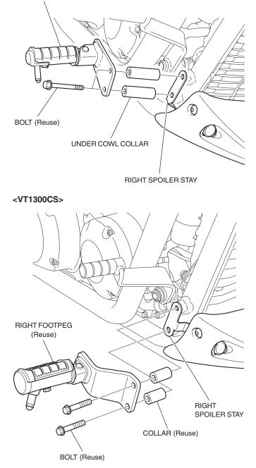
25. Tighten the loosely installed hardware to the torque values specified in the torque chart and Service Manual.
