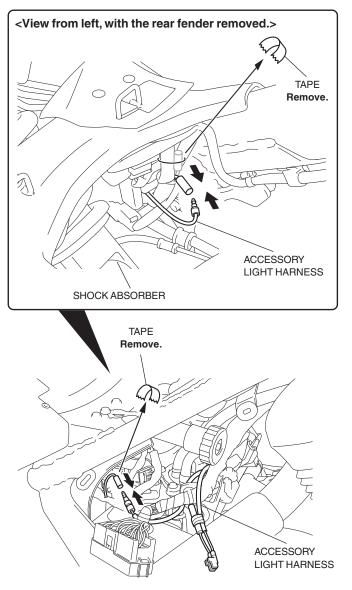
30. Connect the terminal of the accessory light harness to the OP position of the fuse box as shown. Reinstall the fuse box.
