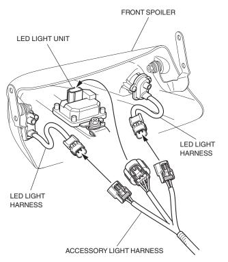
17. Secure the connected accessory light harness with a wire tie as shown.
