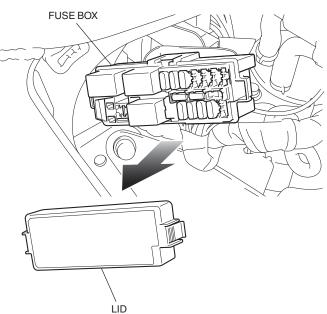
32. Install the 10A fuse in the OP position as shown.
