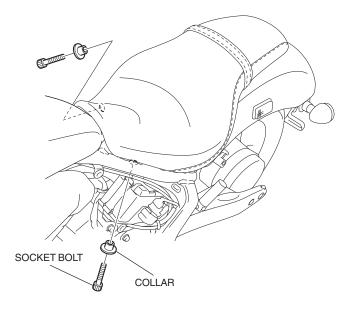
6. Remove the seat from the motorcycle as shown.Applies to VT1300CS only.
