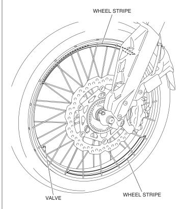
Clean the surface of the area shown using isopropyl alcohol.
