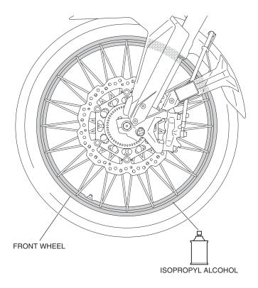
2. Remove the adhesive backing on the front wheel stripe as shown.
