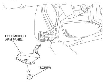
7. Remove the left rear view mirror as shown.
