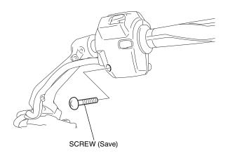
33. Remove the CB switch case as shown.
