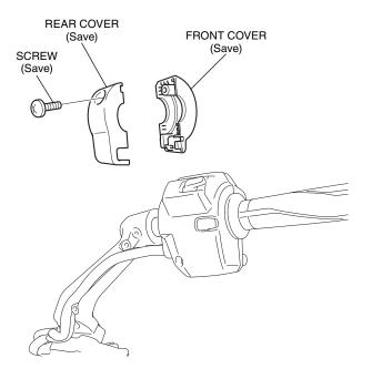
32. Remove the screw as shown.
