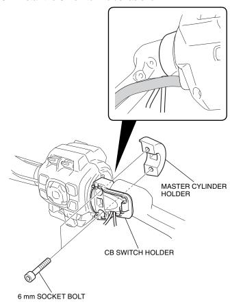
35. Install the CB switch case as shown.
