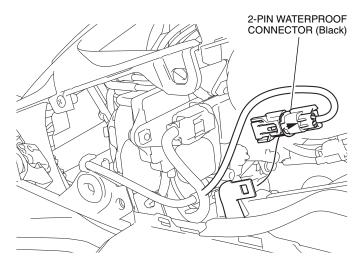
18. Remove the clip and disconnect the connector as shown.
