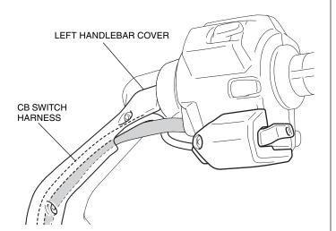
49. Secure the CB switch harness with the wire tie as shown.
