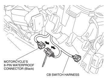
42. Secure the CB switch harness with the holder clip as shown.
