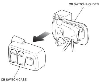
34. Install the CB switch holder as shown.
