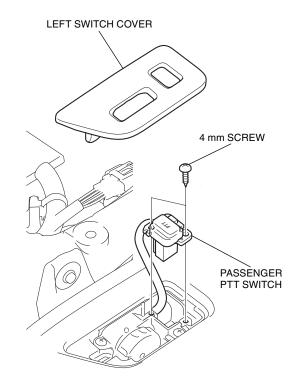
10. Secure the passenger PTT switch harness with the wire tie.
