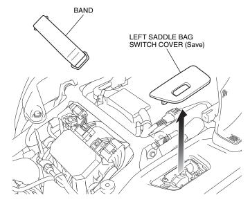
7. Move the rear control unit, and remove the 2P Black dummy connector as shown.
