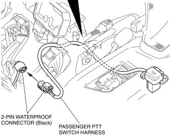
9. Install the passenger PTT switch and left switch cover as shown.
