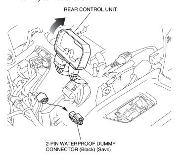
8. Route and connect the passenger PTT switch harness as shown.
