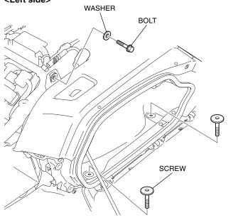
23. Remove the screw as shown.
