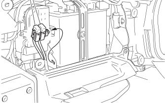
10. Remove the left passenger step holder cover as shown.
