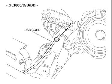
32. Secure the USB cord with the wire tie as shown.
