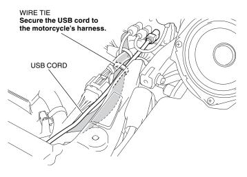
33. Secure the USB cord with the wire tie as shown.
