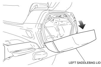
2. Remove the left side cover as shown, and disconnect the negative (-) cable from the battery.
