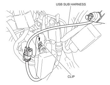
19. Secure the USB sub harness with the wire tie as shown.
